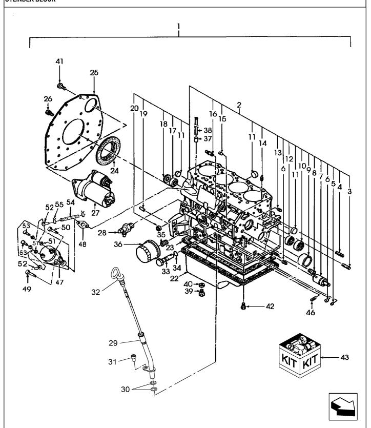
Complete engines are typically not available. Recommendation is to order the Long Block through PAL. Long Blocks as listed in PAL are complete engines less the starter, belts, alternator, flywheel.
